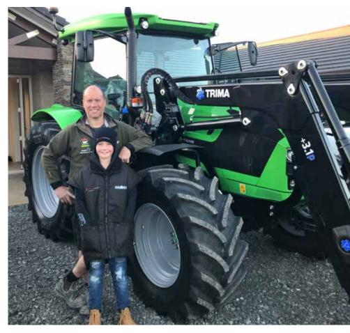
emission regulations. Part of the design sees that engine delivering maximum torque of a rev range from 1,900 down to 1,200 rpm, meaning it offers the ability to 'hang on' as conditions get tough, and remove the need to hunt for gears.
